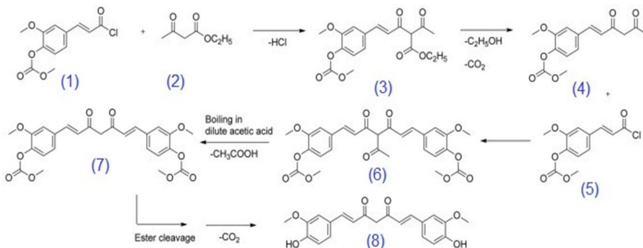
Figure 3. Synthesis of curcumin according to Lampe<sup>[9]</sup>
