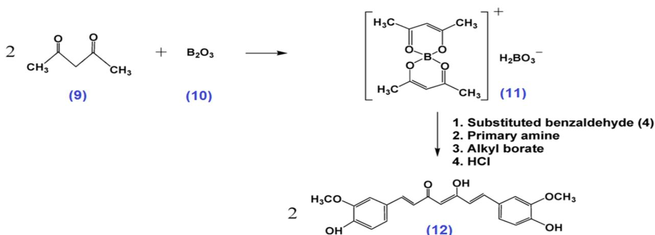
Figure 4. Synthesis of curcuminoids according to Pabon
